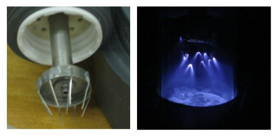
Figure 24. Left, the electrode of the small plasma chamber used in the first study. Right, plasma treatment of sesame seeds – an earlier study. (The chamber holds only seven cotton seeds.)
