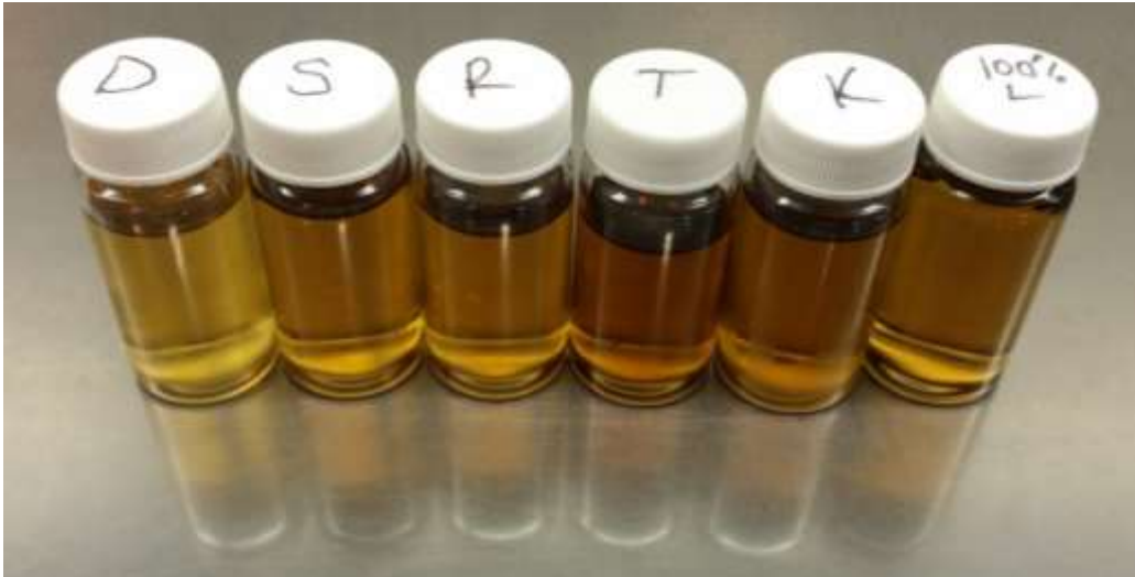
Figure 19 Water extract of stubble varieties (100% of 100g/L) of selected rice varieties (L to R: Doongara, Sherpa, Reiziq, Topaz, Kyeema, and Langi).
