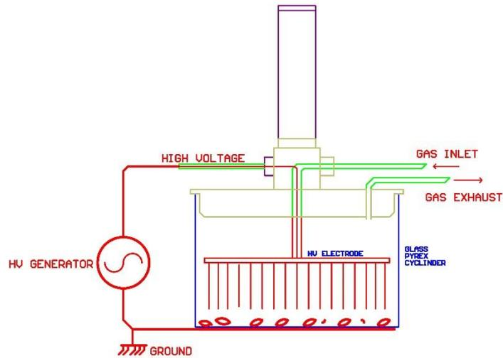
Figure 13. Diagram of plasma chamber used in the second study. Dielectric-barrier discharge treatment chamber, electrode and material exposed to plasma. (The chamber is placed on a shaker – not shown – to ensure rolling and mixing of the seeds during treatment.
