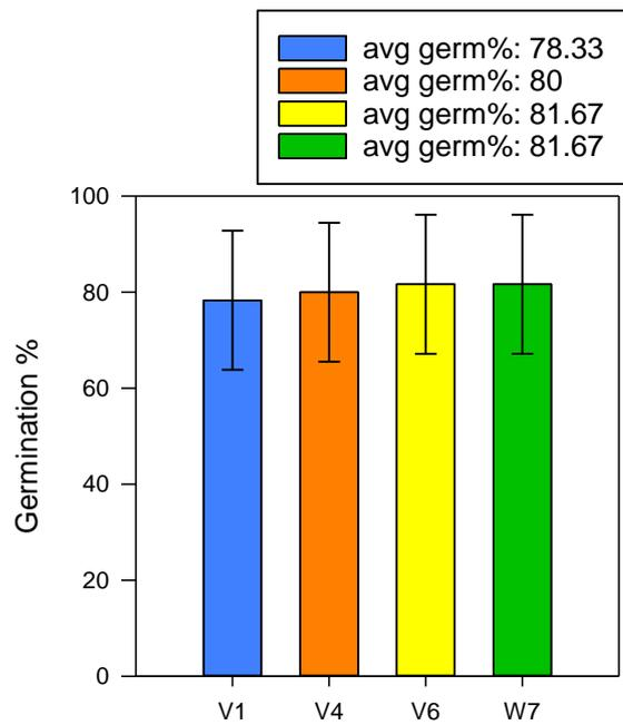
Figure 6: Results of the Imbibitional chill test in Study II. Error bars are twice the LSD (least significant difference) at the 95% confidence interval of the mean. (V1 is control, V4 is 3 min air, V6 is 27 min air, W7 is 81min Argon).
