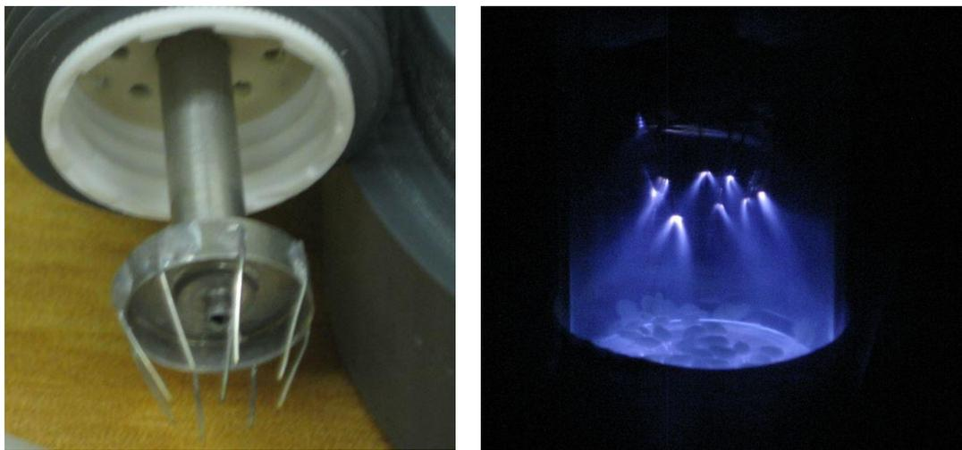
Figure 24. Left, the electrode of the small plasma chamber used in the first study. Right, plasma treatment of sesame seeds – an earlier study. (The chamber holds only seven cotton seeds.)
