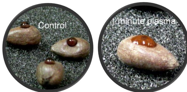
Figure 1. Water drops on plasma treated seeds (using a previous smaller plasma system, not from Study II). The plasma treated surface is more hydrophilic.
