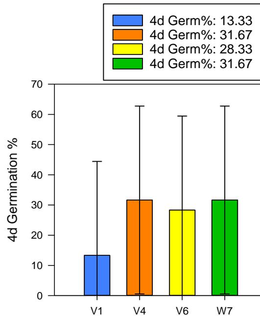
Figure 4: Results of cold germination studies measured at 4 days. Error bars are twice the LSD (least significant difference) at the 95% confidence interval for the mean. (V1 is control, V4 is 3 min air, V6 is 27 min air, W7 is 81min Argon).
